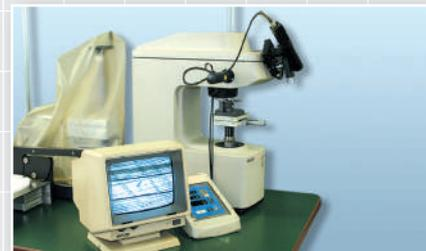
Tester for measuring micro hardness
